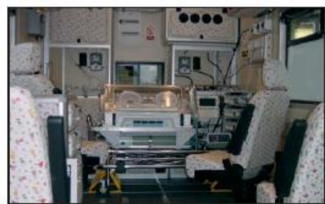
Neonatal transport unit must be secured safely in the ambulance
