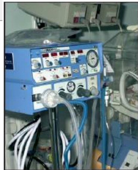
Conventional mechanical ventilators are usually set to deliver a given number of breaths for a set inspiratory time at a set pressure
